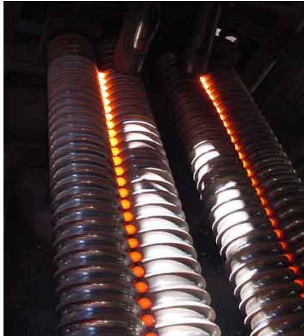
Figure 5. Melted Globes of Glass Being Formed into Marbles [7].
