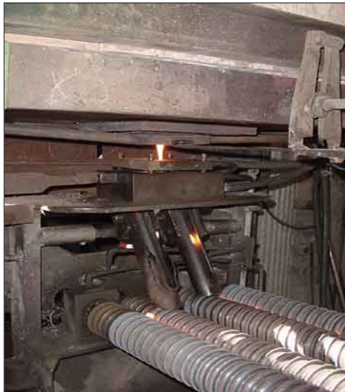
Figure 4. Front of Furnace with Rolling Machine Attached (Jabo Inc. 2003) [7].
