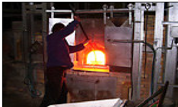
Figure 1. Mixing and Furnace Charging into a Pot Furnace [6].
