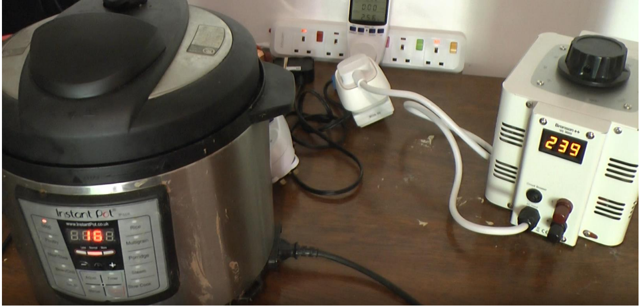
Figure 3 Screen shot of video log of experimentation (From left to right:- Instant Pot (EPC), Nexleaf trekdata logger, Energenie plug monitor, Wemo plug monitor, Variac. Ibutton temperature sensor not shown).
