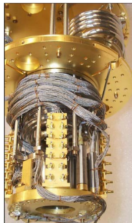
Janis dilution refrigerator with many cables
