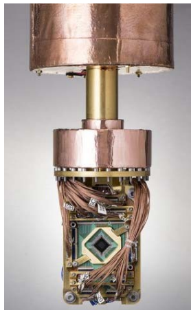
D-Wave processor in a dilution refrigerator (shields removed)
