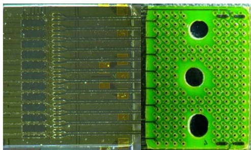
Microscopic images of epoxy underfill process
